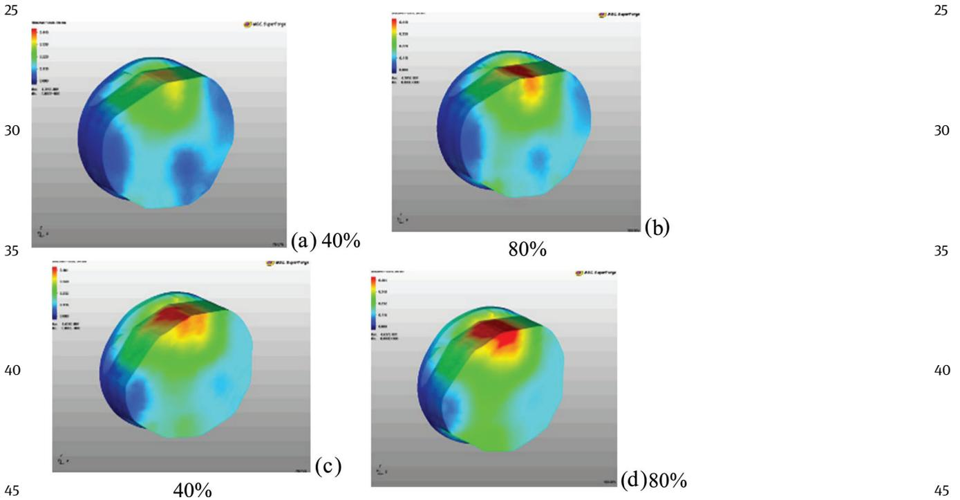
Figure 2 Picture of deformation intensity distribution when forging in the combined baizes with angles of rotation  $30^{\circ}$  (a and b) and  $60^{\circ}$  (c and d),  $t=960^{\circ}\text{C}$
