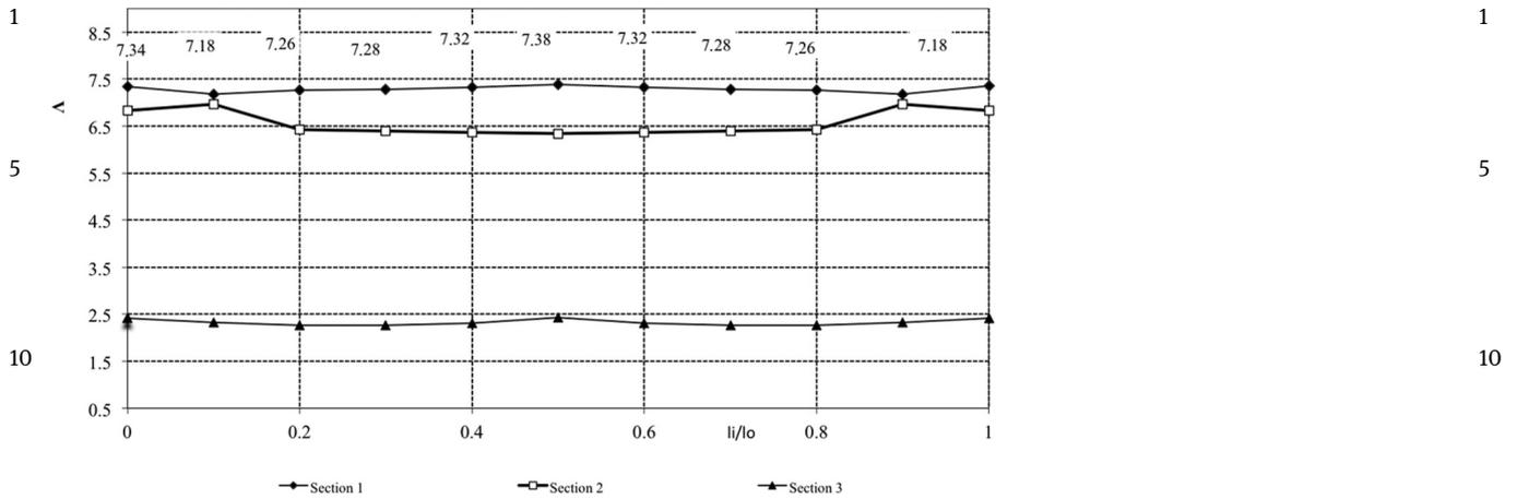
15 **Figure 11** Distribution of  $\lambda$  on the longitudinal section of workpiece at broach on RFM (section 1 –  $D_i/D_0=0.9$ ; section 2 –  $D_i/D_0=0.75$ ; section 3 –  $D_i/D_0=0.5$ ;  $l_i$  and  $D_i$  – distance to a studied point on length and diameter, respectively;  $l_0$  and  $D_0$  – length and diameter of the deformation center, respectively)
