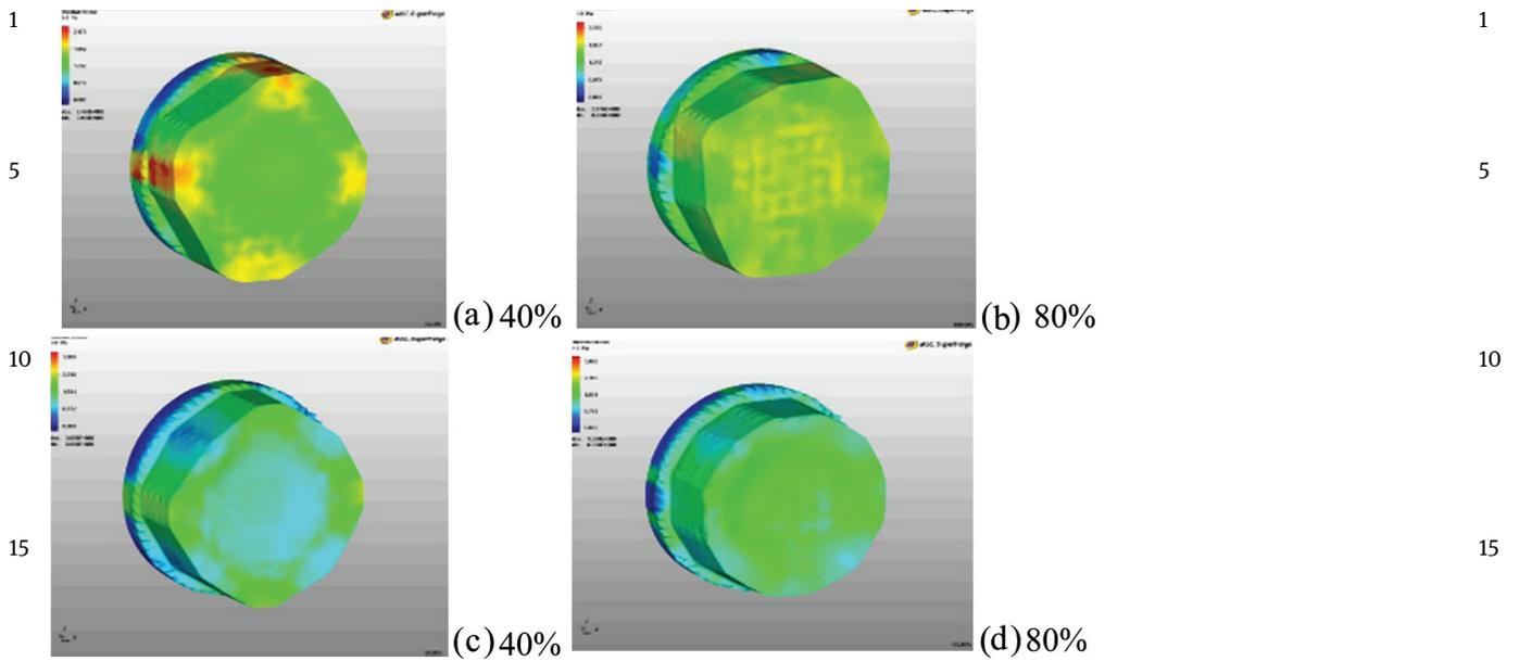
Figure 9 Picture of intensity tension distribution when forging on RFM with angles of rotation 30° (a and b) and 60° (c and d),  $t = 1,150^{\circ}\text{C}$
