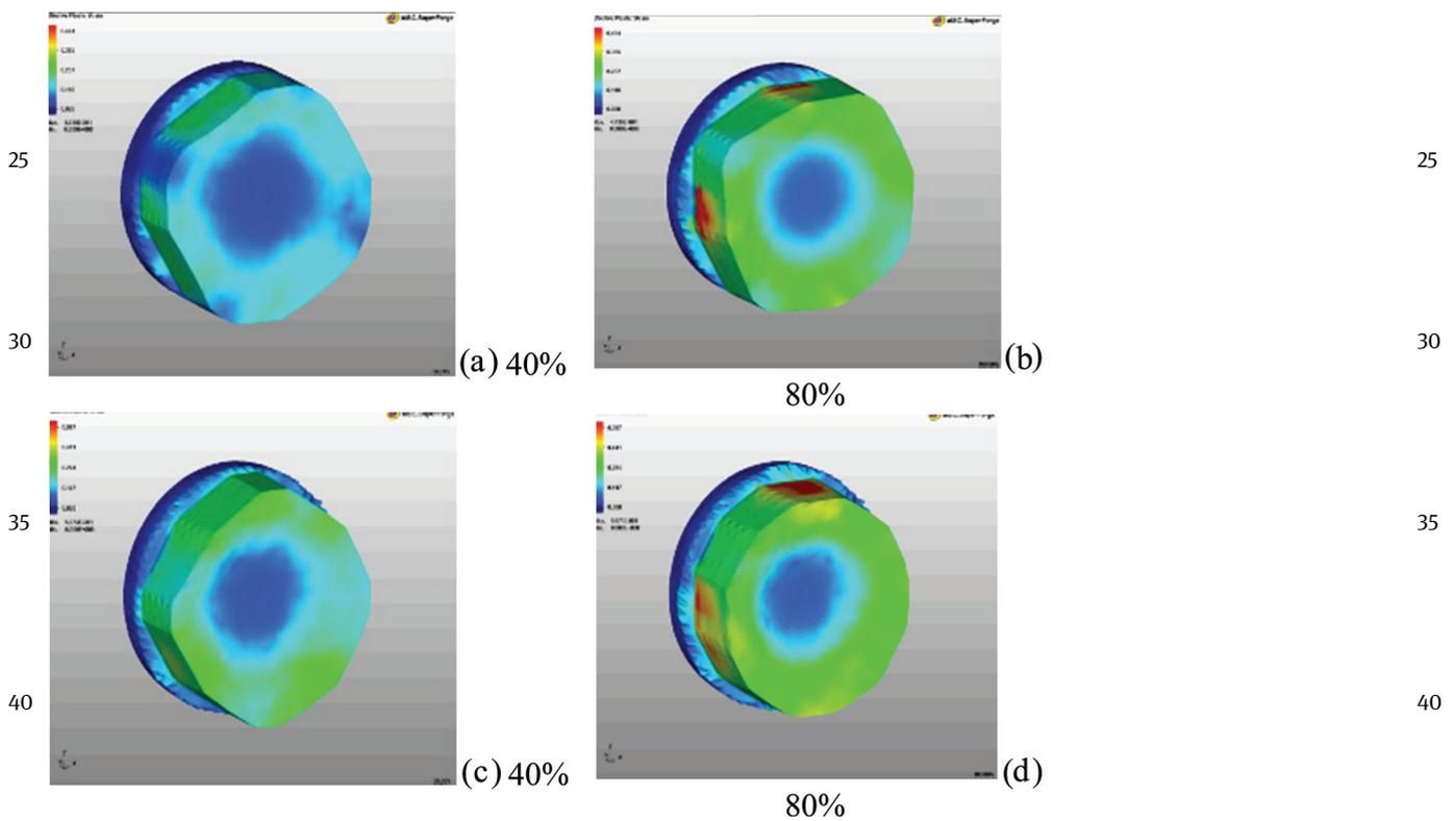
Figure 10 Picture of deformation intensity distribution when forging on RFM with angles of rotation 30° (a and b) and 60° (c and d),  $t = 1,150^{\circ}\text{C}$
