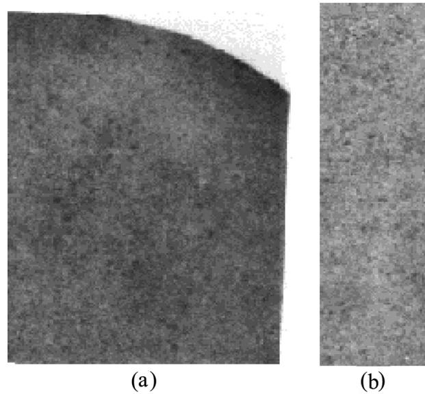
40 **Figure 12** Macrostructure of an alloy of BT9 in cross and longitudinal sections after a broach in flat baizes at temperatures of  $\beta$ -areas, in the combined baizes of  $(\alpha + \beta)$ -areas and on RFM in  $\beta$ -areas
