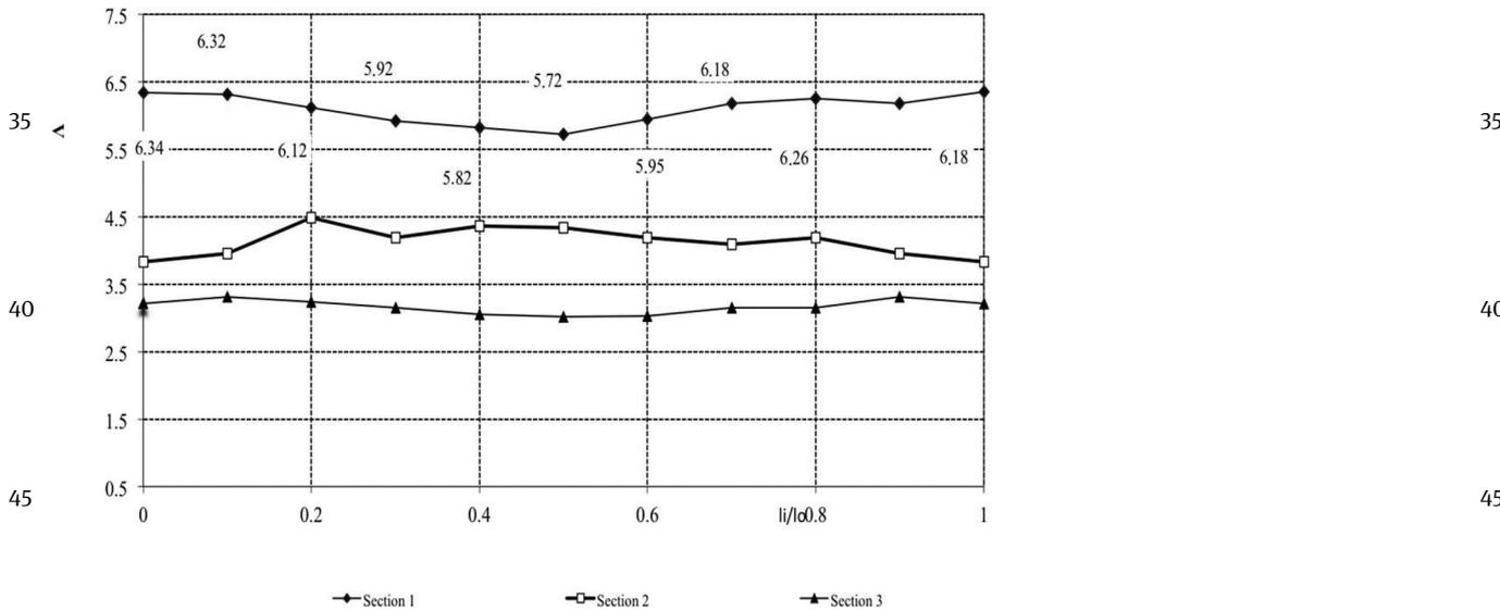
**Figure 4** Distribution  $\Lambda$  on the longitudinal section of workpiece at a broach in the combined baizes with relative giving 0.6 (section 1 –  $D_i/D_0 = 0.9$ ; section 2 –  $D_i/D_0 = 0.75$ ; section 3 –  $D_i/D_0 = 0.5$ ;  $l_i$  and  $D_i$  – distance to a studied point on length and diameter, respectively;  $l_0$  and  $D_0$  – length and diameter of the deformation center, respectively)
