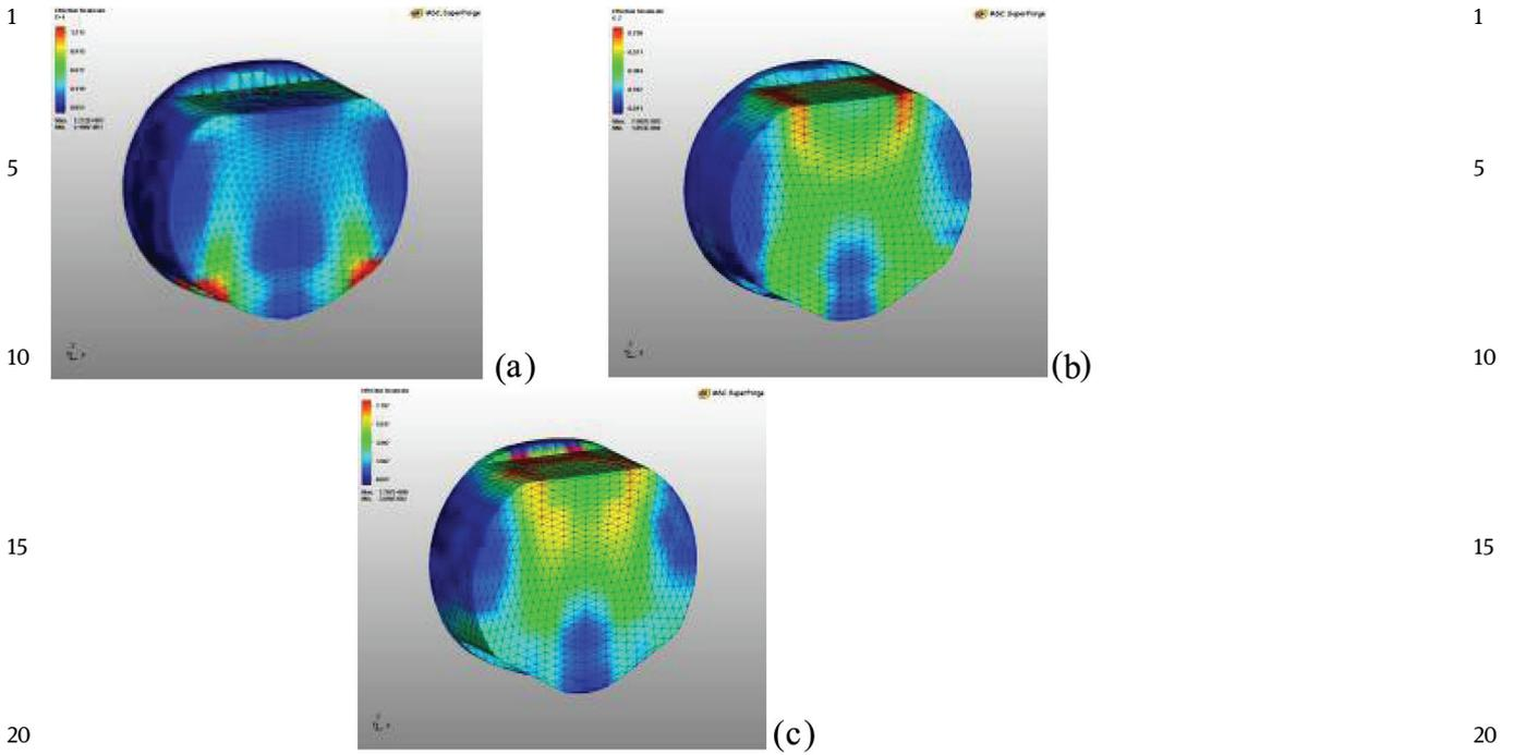
Figure 1 Picture of deformation intensity distribution when forging in the combined baizes with single reduction of 80%,  $t=960^{\circ}\text{C}$ . (a)  $S=1.0$ ; (b)  $S=0.8$ ; (c)  $S=0.6$
