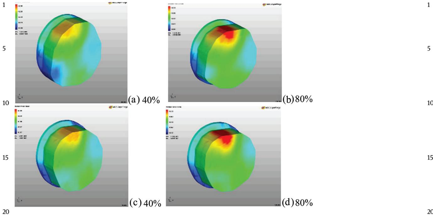
**Figure 3** Picture of deformation intensity distribution when forging in the combined baizes with angles of rotation 90° (a and b) and 120° (c and d),  $t=960^{\circ}\text{C}$
