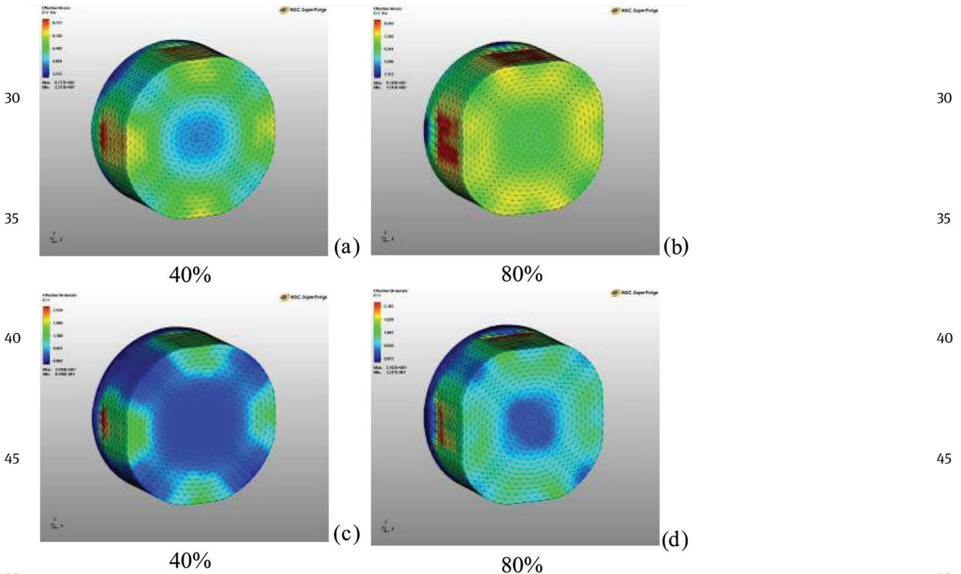
Figure 8 Picture of tension intensity distribution (a and b) and deformations (c and d) in workpiece when forging on RFM,  $t = 1,150^{\circ}\text{C}$
