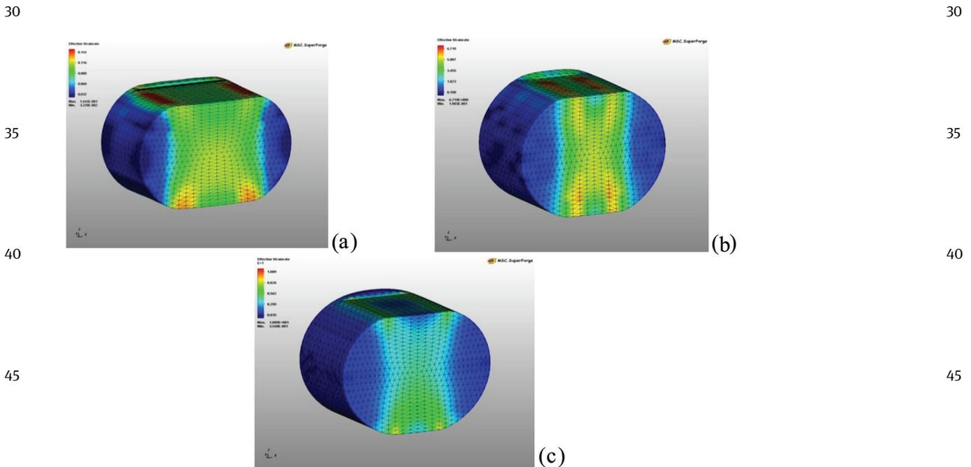
50 **Figure 5** Picture of deformation intensity distribution in workpiece at a broach in flat baizes with single reduction of 80%,  $t = 1,250^\circ\text{C}$ . 50
