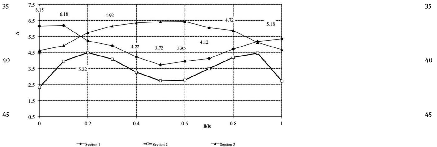
**Figure 7** Distribution of  $\lambda$  on the longitudinal section of workpiece at a broach in flat baizes with relative giving of 1.0 (section 1 –  $D_i/D_0=0.9$ ; section 2 –  $D_i/D_0=0.75$ ; section 3 –  $D_i/D_0=0.5$ ;  $l_i$  and  $D_i$  – distance to a studied point on length and diameter, respectively;  $l_0$  and  $D_0$  – length and diameter of the deformation center, respectively)
