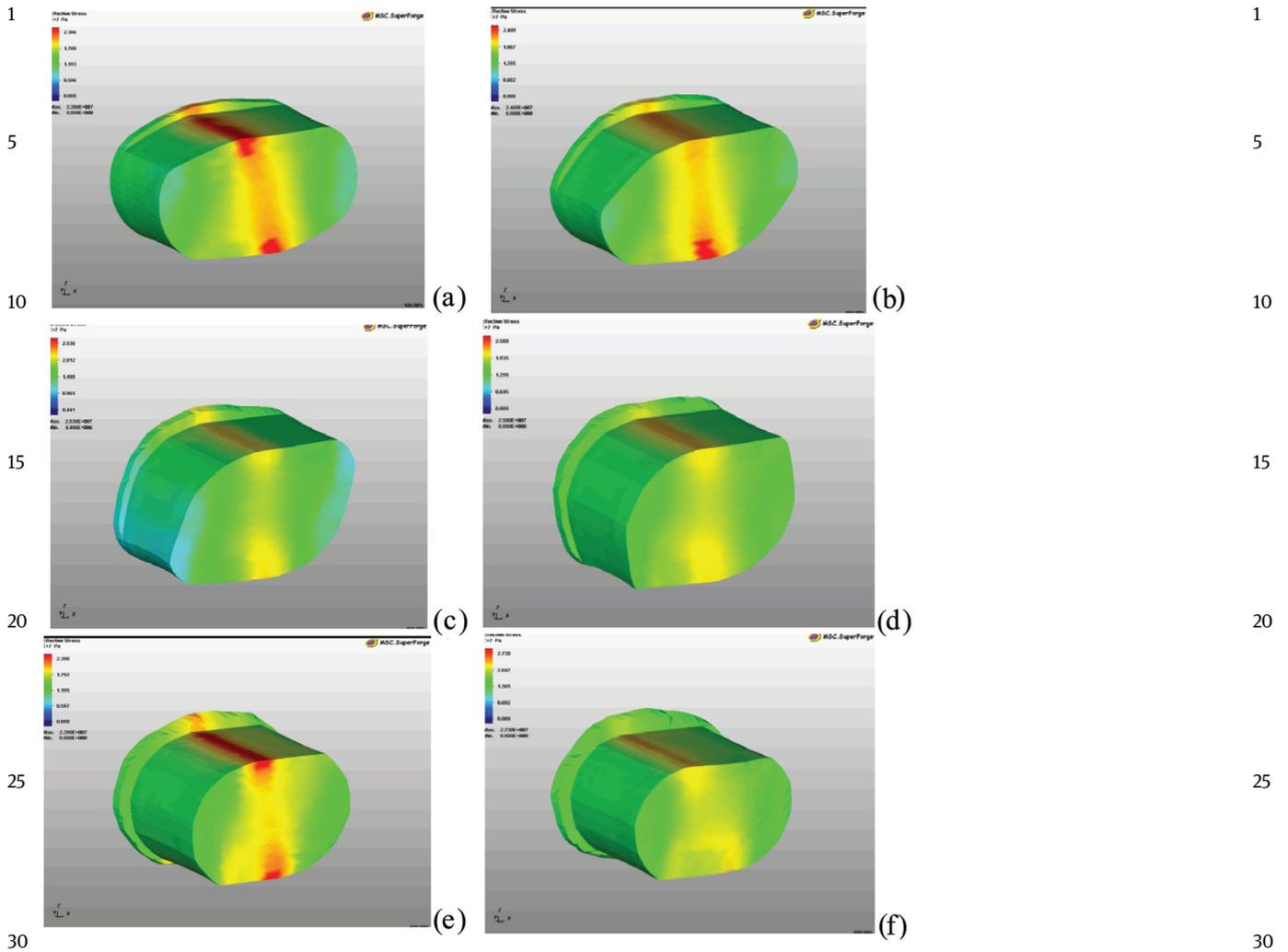
**Figure 6** Picture of deformation intensity distribution in workpiece at a broach in flat baizes with single reduction of 80% and with angles of rotation 30° (a), 60° (b), 90° (c), 120° (d), 150° (e) and 180° (f),  $t=1,250^{\circ}\text{C}$
