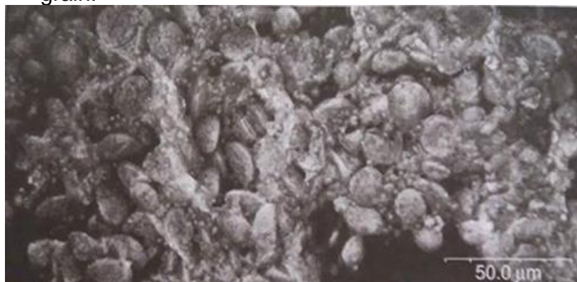
Fig 3. SEM micrograph of triticale starch
