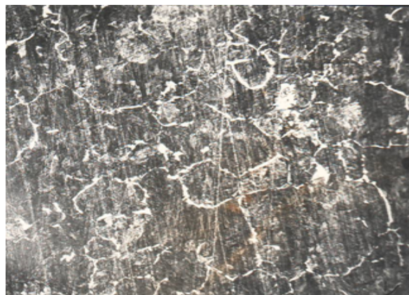
Figure 9. Microstructure of D16 aluminum alloy in the initial state
