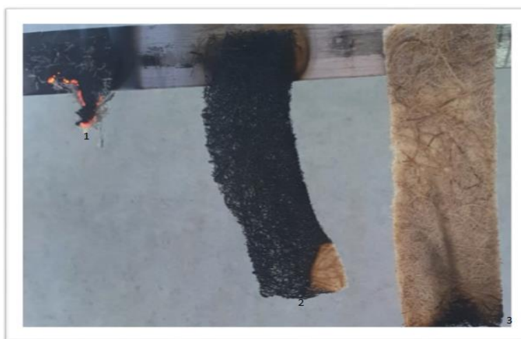
1-sample, raw nonwoven fabric, 2-sample treated with composition: PVA-5 g/l, SP-25 g/l 3-sample treated with composition: GHC-10 g/l, SP-25 g/l
