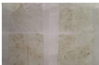
Figure 1 – Cotton fabric processed according to technology 1, after 10 days of microbiological destruction
