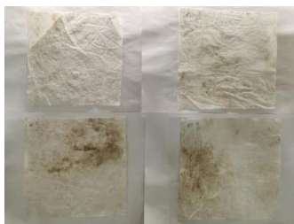
Figure 2 – Cotton fabric processed according to technology 2, after 10 days of microbiological destruction
