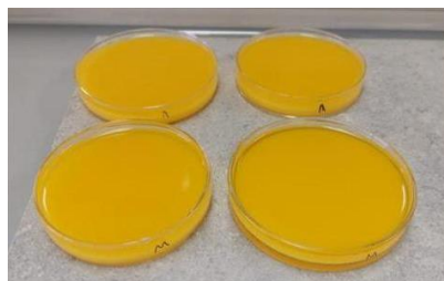
Figure 1 – Preparation of biopolymer based on starch.
