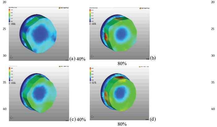
**Figure 10** Picture of deformation intensity distribution when forging on RFM with angles of rotation 30° (a and b) and  $^{45}$  60° (c and d), t = 1,150°C
