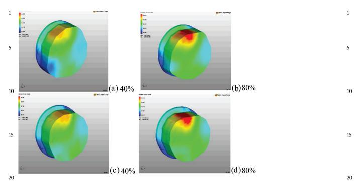
**Figure 3** Picture of deformation intensity distribution when forging in the combined baizes with angles of rotation 90° (a and b) and 120° (c and d), t = 960°C
