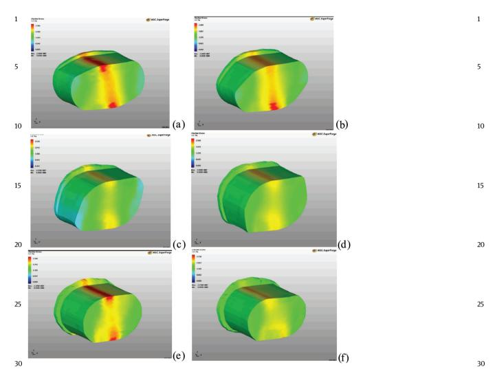
**Figure 6** Picture of deformation intensity distribution in workpiece at a broach in flat baizes with single reduction of 80% and with angles of rotation 30° (a), 60° (b), 90° (c), 120° (d), 150° (e) and 180° (f), t = 1,250°C
