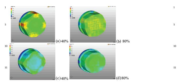
**Figure 9** Picture of intensity tension distribution when forging on RFM with angles of rotation 30° (a and b) and 60° (c and d), t = 1,150°C 20
