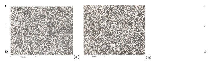
**Figure 13** Microstructure of forgings from BT9 alloy after a broach in  $\beta$ -, ( $\alpha + \beta$ )-,  $\beta$ -areas (a) in the cross section of forging; (b) in the longitudinal section of forging
