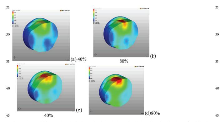
**Figure 2** Picture of deformation intensity distribution when forging in the combined baizes with angles of rotation  $30^{\circ}$  (a and b) and  $60^{\circ}$  (c and d),  $t = 960^{\circ}$ C
