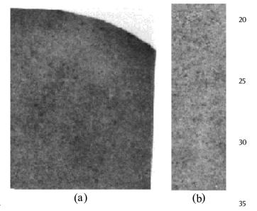
Figure 12 Macrostructure of an alloy of BT9 in cross and longitudinal sections after a broach in flat baizes at temperatures of  $\beta$ -areas, in the combined baizes of ( $\alpha + \beta$ )-areas and on RFM in  $\beta$ -areas
