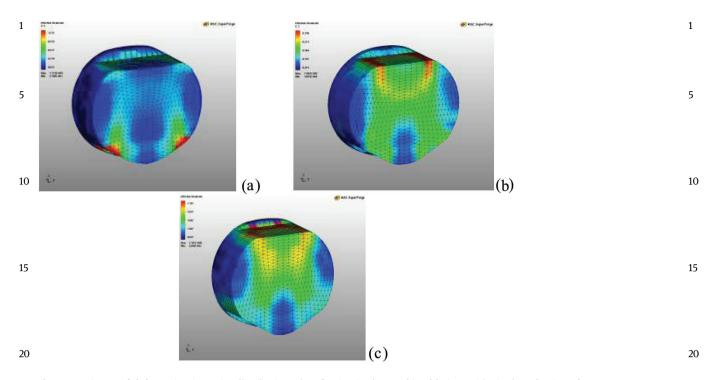
**Figure 1** Picture of deformation intensity distribution when forging in the combined baizes with single reduction of 80%,  $t = 960^{\circ}$ C. (a) S = 1.0; (b) S = 0.8; (c) S = 0.6
