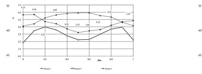
**Figure 7** Distribution of  $\Lambda$  on the longitudinal section of workpiece at a broach in flat baizes with relative giving of 1.0 (section  $1 - D_i/$ 50  $D_0 = 0.9$ ; section  $2 - D_i/D_0 = 0.75$ ; section  $3 - D_i/D_0 = 0.5$ ;  $l_i$  and  $D_i$  – distance to a studied point on length and diameter, respectively;  $l_0$  and 50  $D_0$  – length and diameter of the deformation center, respectively)
