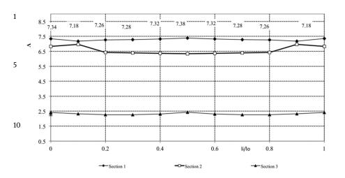
15 **Figure 11** Distribution of Λ on the longitudinal section of workpiece at broach on RFM (section  $1 - D_i/D_0 = 0.9$ ; section  $2 - D_i/D_0 = 0.75$ ; 15 section  $3 - D_i/D_0 = 0.5$ ;  $l_i$  and  $D_i$  – distance to a studied point on length and diameter, respectively;  $l_0$  and  $D_0$  – length and diameter of the deformation center, respectively)
