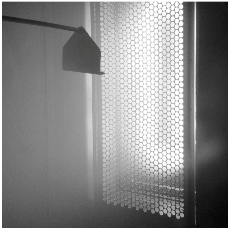
Figure 2: Photograph of the discharge plasma glow inside the chamber at pressure 0.3 Pa of the mixture of argon and nitrogen (15%) and a current in the magnetron target circuit of 8 A
