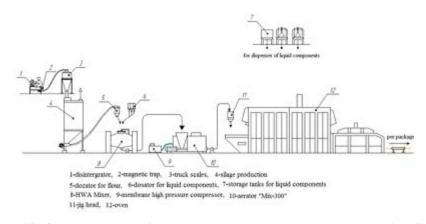
Fig. 2. Production line of whipped bread with phospholipid emulsions of sunflower oil
