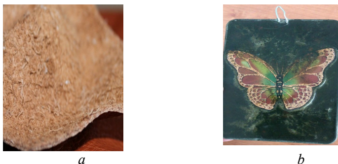
Figure 5 - Samples obtained from powdered leather waste (a-a decorative product in which crushed leather fibers are used as a reinforcing component, b-a sample of artificial material)
